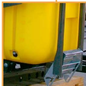
Anti-slip foldable step in order to facilitate the access to the tank opening.
