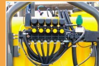
Electric DPM regulator with pressure gauge and remote control box (Adjustable from tractor cabin). Functions +/- pressure, close / opening sections, ON / OFF).
