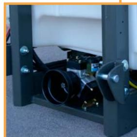
Lower hitch points have different positions in order to suit better to the tractor's geometry.
