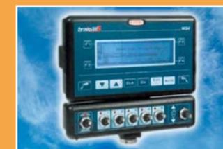
DPAE regulators (computers serie BRAVO) with display and control of different parameters (tractor speed, nozzle flow, L/ha, work pressure...)
