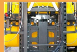
Hydraulic elevation with or without pneumatic suspension (Low pressure air cushions).
