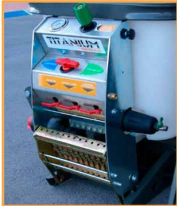
The lateral control panel includes all the functions itself for a simple and easy use. DUAL PRESS system: Auxiliar function pressure is independent from main pressure regulation. Therefore, you can spray at 3 bar meanwhile the agitation works at 10 bar.
