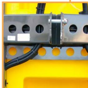
Thanks to plasma cutting and rubber edges, the pipes are well protected inside the frame.
