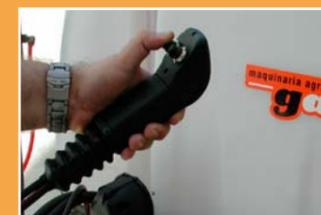
Joystick multifunctions: 2 or 3 buttons. (Fold / Unfold boom, elevation, hydraulic tilt).
