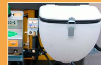
Chemical induction tank (40 litres) with 4 functions: Mixer, fast filling, bottle cleaner and self-cleaning.
